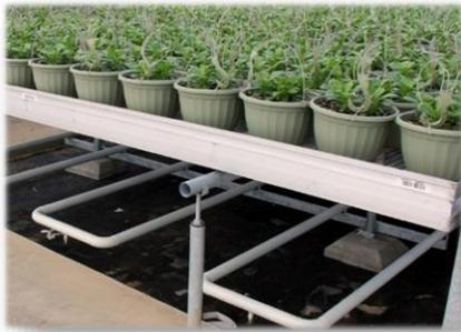
Figure 7: Under bench heating
