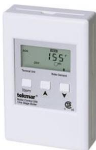
The Tekmar 256 is a boiler controller with outdoor thermometers and warm weather shutdown capability. By monitoring the outdoor temperature and water temperatures in your system it can determine the most appropriate supply temperature and boiler firing rate. This prevents the system from running if the outdoor temperatures are equal or greater than the desired temperature and modulates the burners proportionally to the heat requirement.
